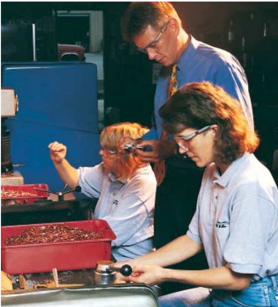
Precise deburring is a critical process for copper chrome zirconium tips. Here, Dave Hinz inspects a tip after it has been deburred.
