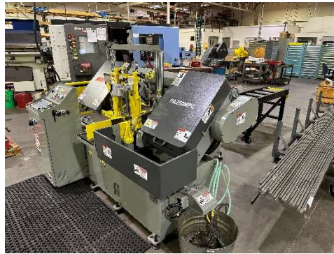
Amada PA260MPC Horizontal Post Style Saw (New 2022)
